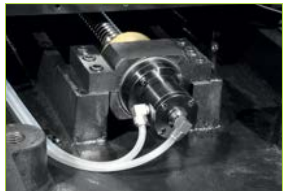
Oil cooling through ballscrew (VF1100, VF1300, VF1500)
